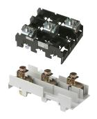
MULTIFIX® 60 is a system for energy distribution comprising a variety of modular combinable components. The energy distribution is carried out via copper bus bars in a 60 mm bus bar system up to 630 A, 400 V AC, 500 V AC, 690 V AC, 45–62 Hz. Short circuit withstand tested to VDE 0660 part 500 and IEC 60439-1.
